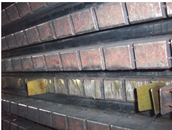
Figure1. Rey 85 MW generator, defects on the tooth of cores.
